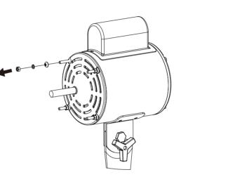
7. Secure the rear guard to the motor and fix it with the bowl washers, flat washers, spring washers and hex nuts removed from step 6.
