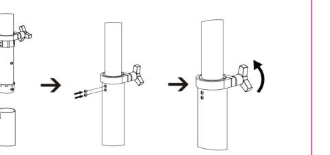
5. Secure the motor to the upper pole and tighten it with the locking screws provided.
