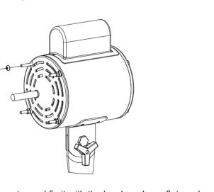
Position guard hooks of front guard into ribs of rear guard.
