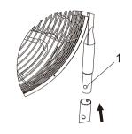
1. Press the buttons (1) on each side of  $_{\perp}$  2. Insert the fan onto the bracket (2) until the buttons snap into place in the bracket.
